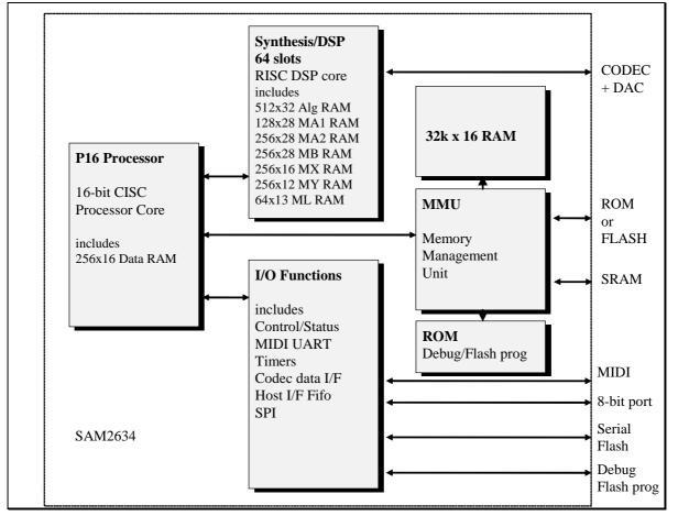
The SAM2634 is a low cost derivative of the SAM2000 series. It retains the same high quality synthesis with up to 64 voices polyphony. The SAM2634 maximum wavetable memory is 32 MBytes and the parallel communication is through a standard 8-bit port. The integrated 32kx16 RAM allows for high quality effects without additional component.
