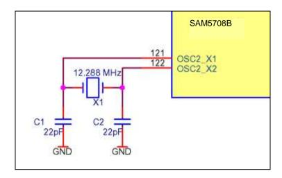
C1 and C2 should be chosen in range 12pF-27pF. Different values lead to different oscillation characteristic and can be selected based on board layout considerations. External feedback resistor should be avoided because there is an internal feedback resistor.
