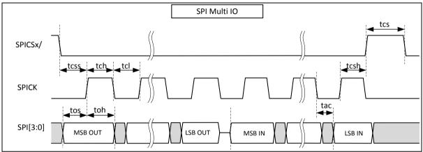
The QSPI controller works on SysClk (usually 196.608MHz with Xtal = 12.288MHz). SPICK frequency is SysClk/Nq. Nq can be programmed between 2 and 4096.
